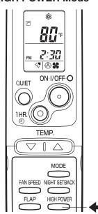
HIGH POWER mode can be used to increase the output of the indoor unit for all operation modes except automatic operation.
